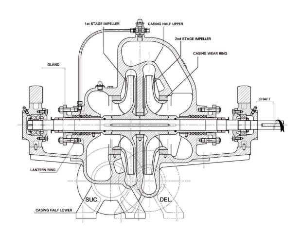
DSM (Thru Bore) Pump with Mechanical - Seal Arrangement
